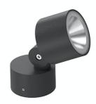
LED source included. LED module configured to work directly on the mains 220-230V ON/OFF. Fixing bracket included. IP68 connector for 6mm<ø<8mm rubber cable. To ensure the tightness of the cable guide it's recommended to use flexible electric cables suitable for exterior use. Ground spike to be ordered separately.
