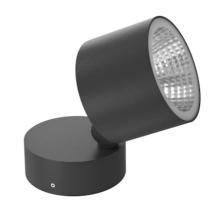
LED source included. LED module configured to work directly on the mains 220-230V ON/OFF. Fixing bracket included. IP68 connector for 6mm<ø<8mm rubber cable. To ensure the tightness of the cable guide it's recommended to use flexible electric cables suitable for exterior use. Ground spike to be ordered separately.
