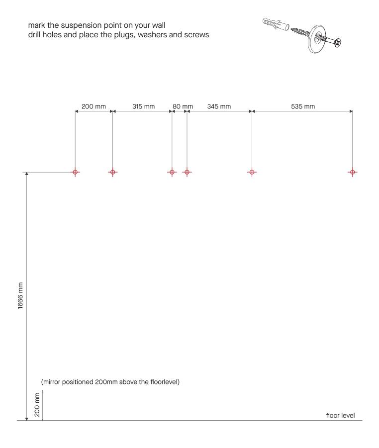
place the mirrors on the washers in the 'open' position
