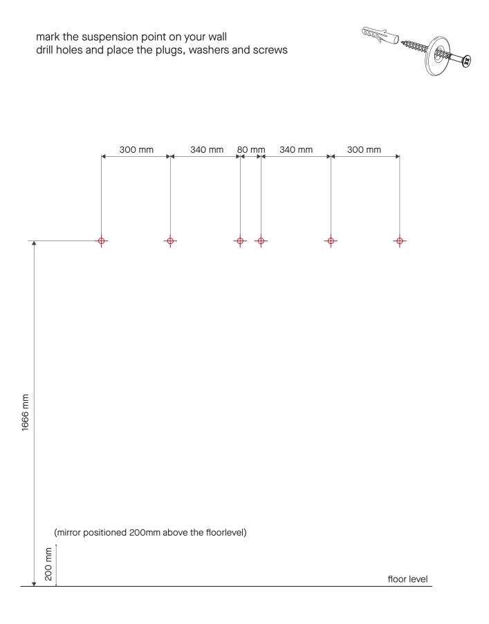
place the mirrors on the washers in the 'open' position
