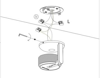
Connect the cables from both the lamp and the mains power into the terminal as illustrated above.
