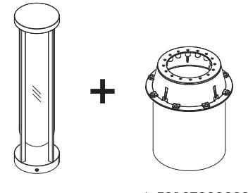
**OPTION 2** con cassaforma - with box for ground installation
