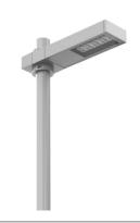
LED source included. Integrated power supply 220-240V ON/OFF and dimmable 1-10V or DALI. Fixing bracket included. Equipped with a 400mm protruding neoprene cable section and IP68 connectors. Single socket for 76mm diameter post. The post must be ordered separately. Smart-City version available upon request.
