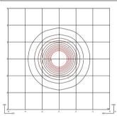
26.94 lm/W Efficiency CG Coordinate System 592.57 lm **Total Flux** Maximum Value 201.28 cd
