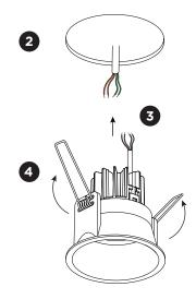
Power must be turned off before connecting the cables.
