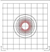
Efficiency Coordinate System 26.935 lm/W CG 593 lm **Total Flux** Maximum Value 201.28 cd
