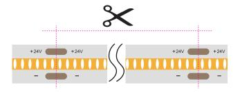
When cutting the strip it is important to cut precisely between 2 LEDs. When an LED is exposed there is no phosphor covering the side which will show blue light coming out of the cut side of the strip.
