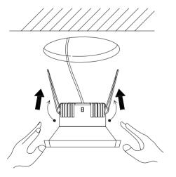
Pull the spring upward, then put the lamp body into the hole and release it
