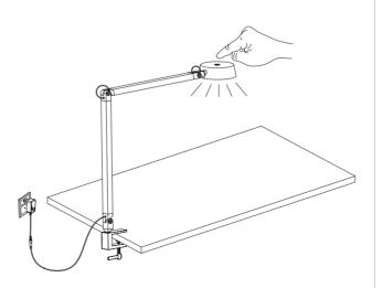
Install the clamp on the table, plug in the power, touch the center of the lamp holder to light up, long press to adjust brightness.
