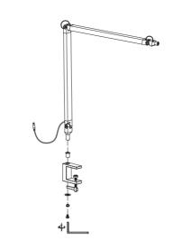
Install the lamp body, plastic cover, clamp, flat gasket, spring
