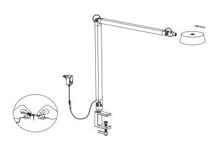
A: Insert the lamp head into the lamp body.
