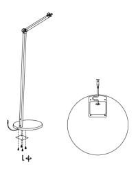
Clip the wire into the base slot and cover the wire with the bottom plate. Then use 2.5\*2.5mm 7 spanner to lock M4 screw into bottom plate.
