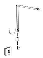
Install the lamp body, plastic cover, wall mount, flat gasket, spring washers, cylindrical head hexagon screws, with 5mm spanner to lock them successively.
