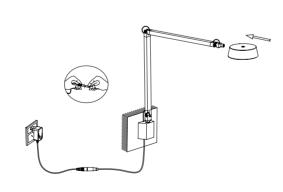
Insert the lamp head into the lamp body
