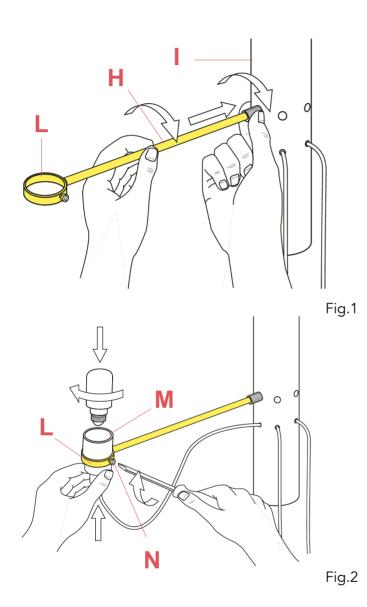
Screw the arms (H) to the lamp body (I), taking care not to bend on the rings (L). Insert the lamp holder (M) in the ring (L) and fasten them by locking the screw (N).
