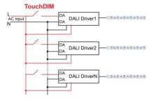
Remark: Only use open push button without indicator light. Maximum cable length between each Unit: 20 meters.
