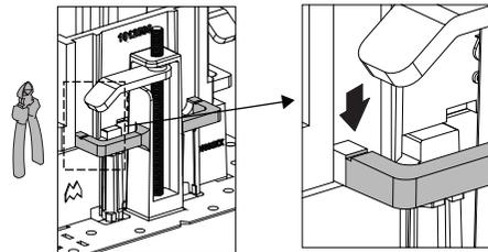
STEP 4: BREAK-OFF THE FLANGES ON THE CORRECT BREAK-OFF LINES
