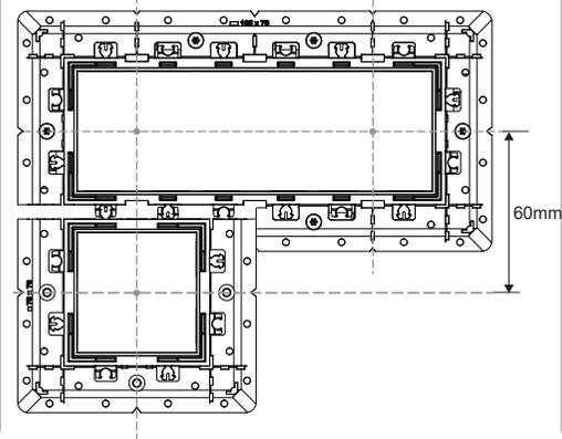
STEP 7: INSTALL THE FRAME BY USING INSTALLATION INSTRUCTION
