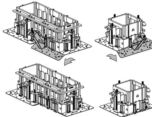
STEP 5: CONNECT THE FRAMES BY PRESSING THE SNAP FEATURES INTO EACH OTHER
