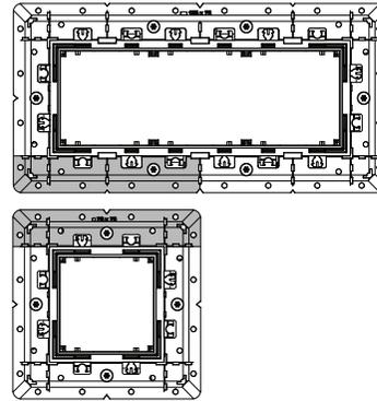
STEP 3: USE SIDE CUTTER TO CUT LOOSE CORRECT REINFORCEMENT ARMS ON THE CUT MARKER
