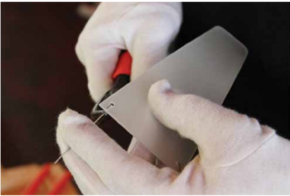
Figure 0.8 Use points of pliers at glass edge.
