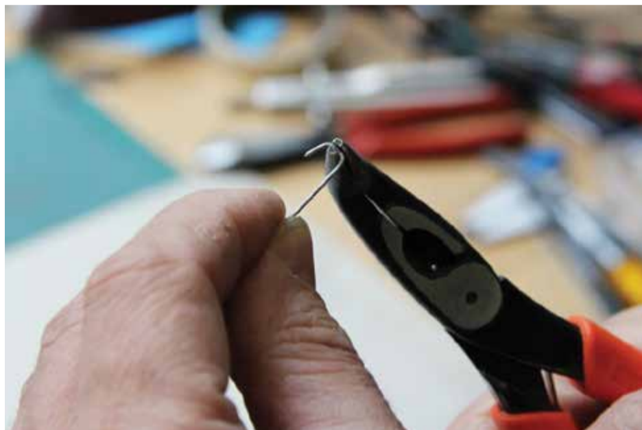
Figure 0.3 Second bend to complete a hook.
