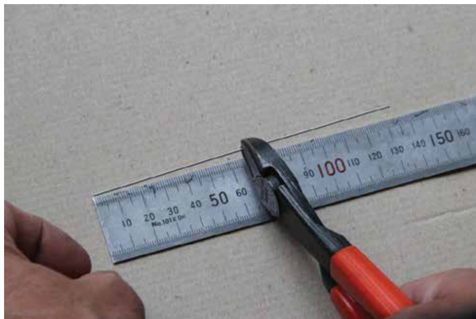
Figure 0.1 Cut the provided wire (130mm) in half (65mm). Side cutters (A).
