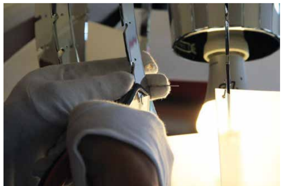
Figure 1.5 Adjust glass so it is seated at base of slots, use pliers to pull wire into leg and bend tightly around the back.
