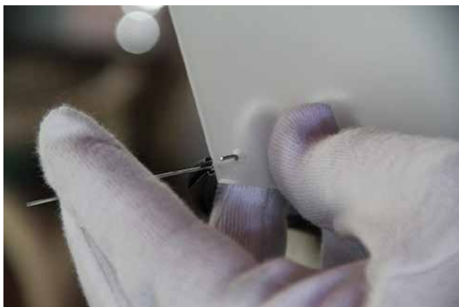
Figure 0.7 Pull wire with index and second finger.
