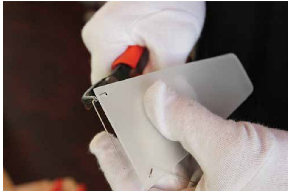
Figure 0.9 Bend wire sharply over the pliers as shown. Repeat on other side.
