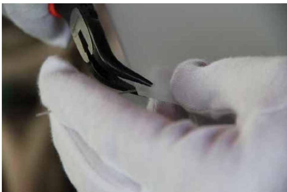
Figure 0.6 Carefully pinch the wire across the hole to tighten it.
