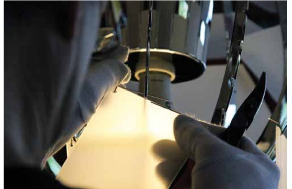
Figure 1.3 Tilt glass and feed left straight wire through hole in leg.
