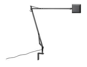
Adjustable table lamp providing direct light. Aluminium painted or chromed body, with die cast head, joints and forks, and extruded arms. Diffuser in photoengraved polycarbonate and aluminate on the perimeter. Edge Lighting technology light source. Optical switch sensor placed on the head that provide 3-step dimming function and color temperature adjustment at 2700K or 3200K. Power cord length 150 cm. Plug-in power supply with interchangeable plugs.
