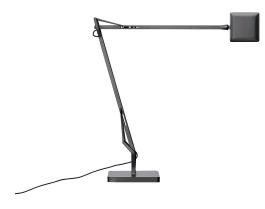
extruded arms. Diffuser in photoengraved polycarbonate and aluminate on the perimeter. Edge Lighting technology light source. Optical switch sensor placed on the head that provide 3-step dimming function and color temperature adjustment at 2700K or 3200K. Power cord length 150 cm. Plug-in power supply with interchangeable plugs.
