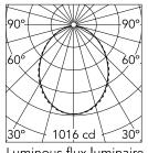
Luminous flux luminaire 2364 lm
