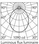
Mountings Ground LED Lamp category Power (W) 30 4000K Colour temperature **CRI** 80 2760 lm Lumen Voltage (V) 230 **Environment** Outdoor
