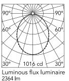
Mountings In-ground Lamp category LED Power (W) 30 Colour temperature 2700K 80 **CRI** 2490 lm Lumen Voltage (V) 230 **Environment** Outdoor
