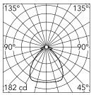
Luminous flux luminaire 2400 lm
