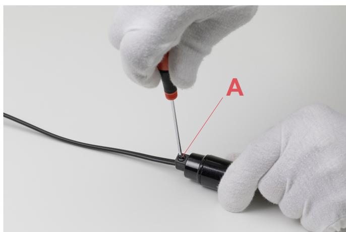
Loosen the screw (A) of the cable clamp on the spare-part kit and also the one present on the lamp fixture.
