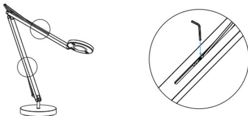
The lamp head joint can be readjusted using a small screw. To do this, carefully remove the cover plate over the joint and slightly tighten the screw with the allen key provided. Then replace the cover plate over the joint.
