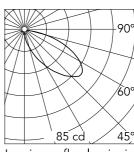
Beam Angle: 45° E(Ix) D(m) h(m) 2.68 1 85 2 5.36 21 3 9 8.04 4 5 10.71 5 3 13.39
