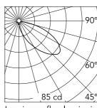
Beam Angle: 45° E(Ix) D(m) h(m) 2.68 85 1 2 5.36 21 3 9 8.04 4 5 10.71 5 3 13.39
