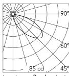
Beam Angle: 45° E(Ix) D(m) h(m) 2.68 1 85 2 5.36 21 3 9 8.04 4 5 10.71 5 3 13.39
