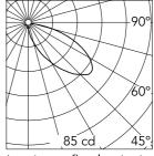
Luminous flux luminaire 266 lm
