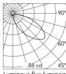
Beam Angle: 45° E(Ix) D(m) h(m) 2.68 1 88 2 5.36 22 3 10 8.04 4 6 10.71 5 4 13.39
