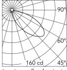
Luminous flux luminaire 503 lm
