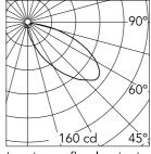
Luminous flux luminaire 503 lm
