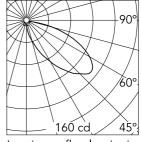
Luminous flux luminaire 503 lm
