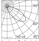
Luminous flux luminaire 503 lm
