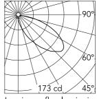
Luminous flux luminaire 543 lm
