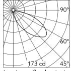
Luminous flux luminaire 543 lm
