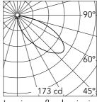
Luminous flux luminaire 543 lm
