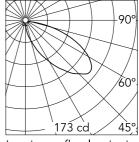
Luminous flux luminaire 543 lm
