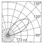
Luminous flux luminaire 543 lm
