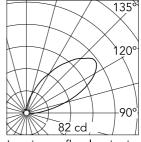
Luminous flux luminaire 256 lm
