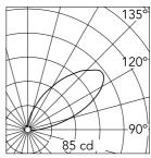
Luminous flux luminaire 266 lm
