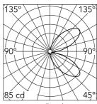
Luminous flux luminaire 532 lm
