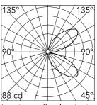
Luminous flux luminaire 554 lm
