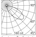
Luminous flux luminaire 503 lm
