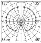
Luminous flux luminaire 1400 lm
