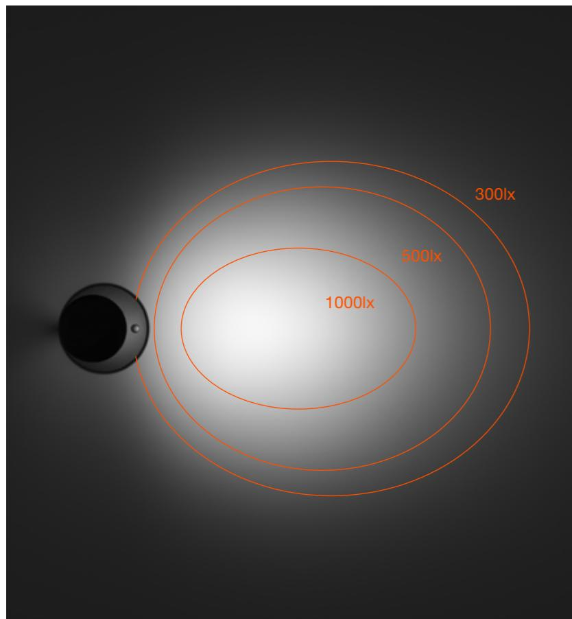
The excellence of comfort: UGR is lower than 10 for an exceptional anti-glare protection, homogeneity of light distribution and lux performance, in accordance to the strictest industry standards.
