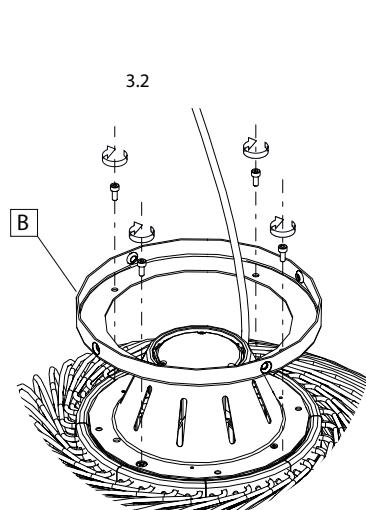
EN 3.2 Position and fasten the bottom part of the junction ring (B) on top of the lower structure (III) using 4 screws.
