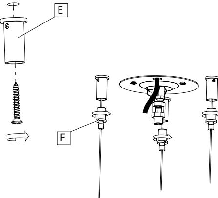
**EN** Install the base of the suspension cable clips (E) using screws, and then attach the adjustable elements of the cable clips (F).
