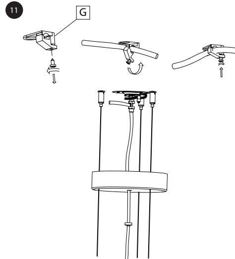
**EN** Fasten the cable clip (G) over the electrical cable.
