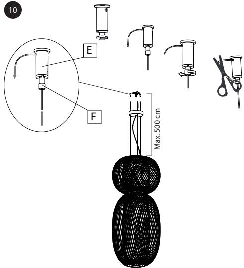
**EN** Feed the steel suspension cable through the cable clips (E), set the height of the pendant lamp as required and fix the adjustable element (F) to lock the length of the suspension cable. Cut any excess suspension cable.
