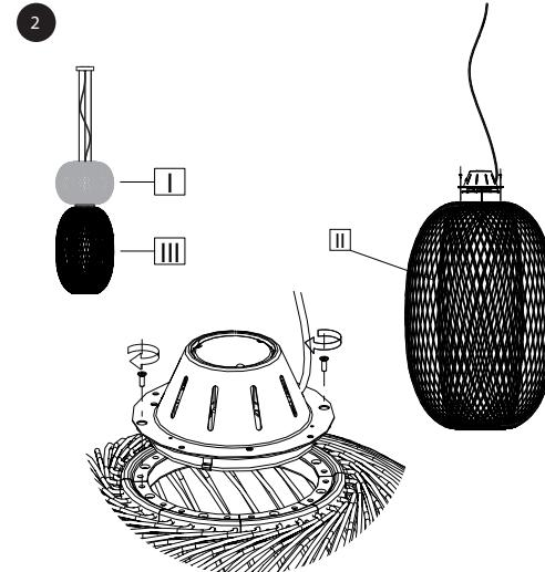
EN On top of the lower structure (III), position and fasten the electrical fitting (II) with two screws.
