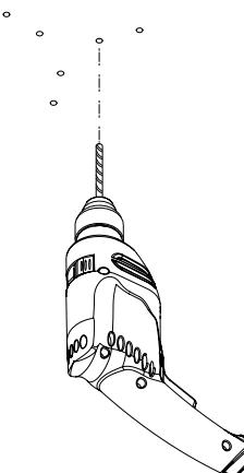
**EN** Using the template supplied, mark out the points on the ceiling for the holes to be drilled.
