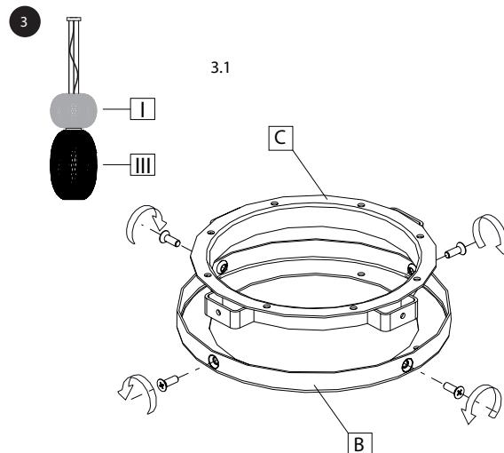
EN 3.1 Disassemble the junction ring (B+C) by removing the screws.
