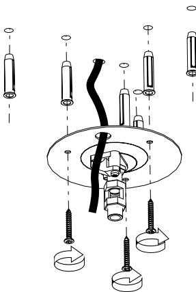
**EN** Install the screw anchors and fix the ceiling mounting plate using screws.
