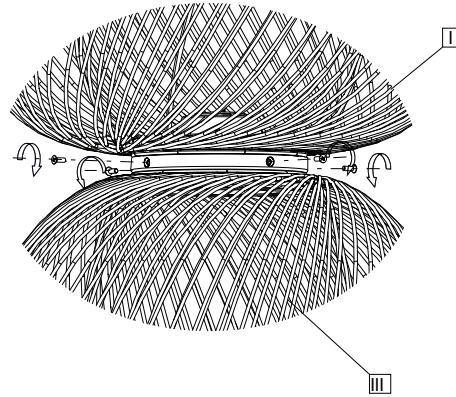
**EN** Feed the electrical cable through the upper structure (I) and fasten the lower (III) and upper (I) structures together at the junction ring using 4 screws.
