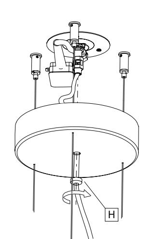
EN Fit the ceiling rose over the mounting bracket and secure it with the knurled screw (H).
