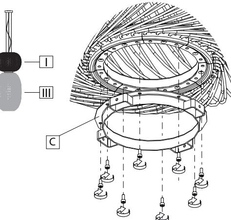
**EN** Position and fasten the upper part of the junction ring (C) on the bottom of the upper structure (I) using 8 screws.
