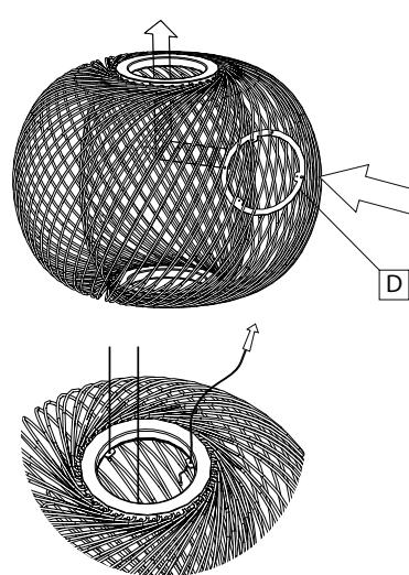
**EN** Insert the suspension ring (D) into the upper structure (I) and fasten it to the underside of the top using 4 screws. Introduce the hanging wires.
