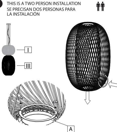
EN Insert the ring (A) into the base of the lower structure (III) and fasten it with two screws.
