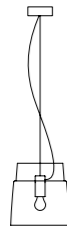
S3 Ceiling Rose Ø 120 mm Cable 2000 mm Diffuser Ø 300 mm H 320 mm
