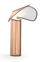
Table lamp composed of a reflecting body in aluminium in 3 colour variations, finished internally with an opaque white plastic film and folded and closed via hooks riveted to the sheet metal. A coloured seal in moulded tpu runs along the entire profile of the body. The internal base in extruded aluminium is attached to the body for stability and it also supports the bulb socket. The power cable has a dimmer switch to adjust the brightness. Usable cable length: 1.9 m
